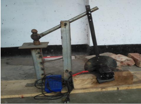
Fig 3: Fabricated Automatic Portable Hammering Machine
